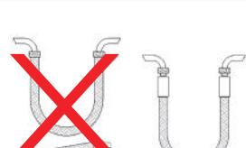
If torsion can not be avoided, use movable couplings which absorb torsion. Thus the hose is only exposed to bending load.
