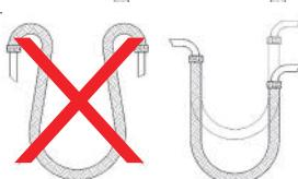
Correct installation only with rigid pipe elbow.
